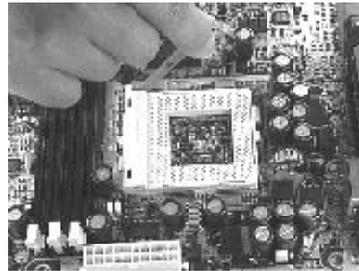
Insert the CPU into the socket. Please keep the lever right angle when inserting CPU.
