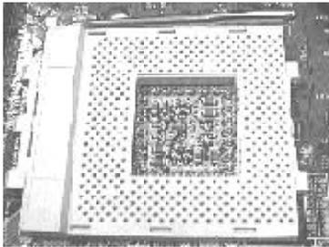
Locate the ZIF socket and open it by first pulling the lever of socket upward.
