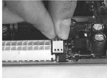
Finally,attach the fan cable to the CPU fan header FCPU.
