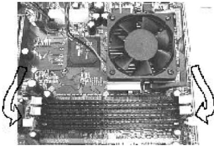
Open latches of DIMM socket.
