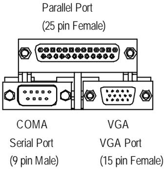
➤ This connector supports 1 standard COM port , 1 Parallel port and 1 VGA port. Device like printer can be connected to Parallel port ; mouse and modem etc can be connected to Serial ports.
