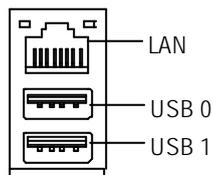
➤ Before you connect your device(s) into USB connector(s), please make sure your device(s) such as USB keyboard, mouse, scanner, zip, speaker...etc. Have a standard USB interface. Also make sure your OS (Win 95 with USB supplement, Win98, Windows 2000, Windows ME, Win NT with SP 6) supports USB controller. If your OS does not support USB controller, please contact OS vendor for possible patch or driver upgrade. For more information please contact your OS or device(s) vendors.
