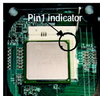
2. Locate Pin 1 in the socket and look for a (golden) cut edge on the CPU upper corner. Then insert the CPU into the socket.
