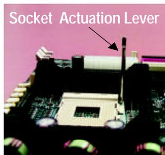
1. Pull up the CPU socket lever and up to 90-degree angle.
