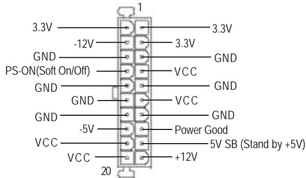
➤ AC power cord should only be connected to your power supply unit after ATX power cable and other related devices are firmly connected to the mainboard.
