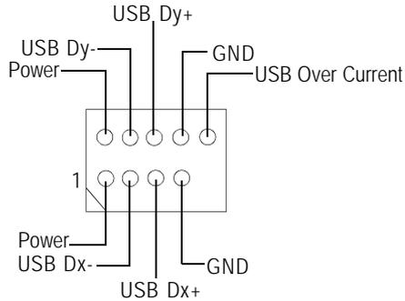
➤ Be careful with the polarity of the front panel USB connector. Check the pin assignment while you connect the front panel USB cable. Please contact your nearest dealer for optional front panel USB cable.
