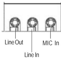
➤ After install onboard audio driver, you may connect speaker to Line Out jack, micro phone to MIC In jack. Device like CD-ROM , walkman etc can be connected to Line-In jack.
