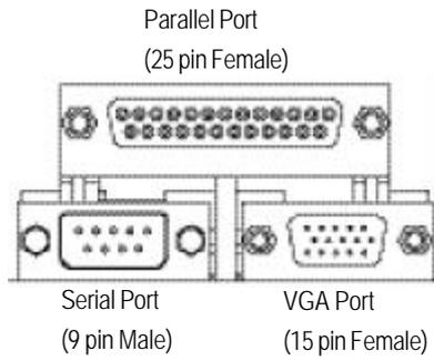
➤ This mainboard supports 1 standard COM port, 1 VGA port and 1 LPT port. Device like printer can be connected to LPT port ; mouse and modem etc can be connected to COM port.
