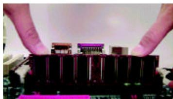
1. The DIMM slot has a notch, so the DIMM memory module can only fit in one direction.
