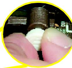
Please carefully pull out the small white-drawable bar at the end of the AGP slot when you try to install/ Uninstall the AGP card. Please align the AGP card to the onboard AGP slot and press firmly down on the slot. Make sure your AGP card is locked by the small white-drawable bar.
