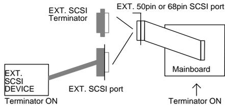
**CASE 2: BIOS SETUP (SCSI Terminator Enable: High Byte)**
