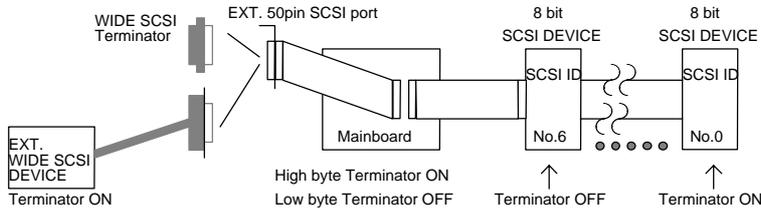
**CASE 3: BIOS SETUP (SCSI Terminator Enable: None)**
