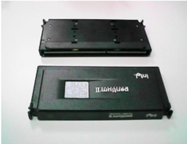
Figure 2:OEM Pentium® II Processor
