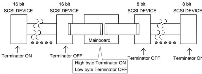
② System has 8 bit EXT. SCSI port & 8 bit INT. SCSI device
