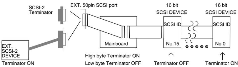
④ System has 16 bit EXT. SCSI port & 8 bit INT. SCSI device
