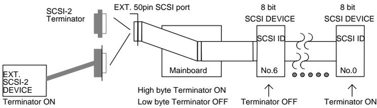
③ System has 8 bit EXT. SCSI port & 16 bit INT. SCSI device
