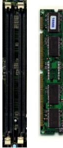
*Insert DIMM into the DIMM sockets at a 90 degree angle.*
