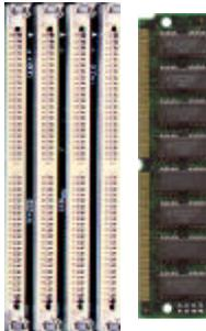
*Insert SIMM into the SIMM sockets at a 45 degree angle.*
