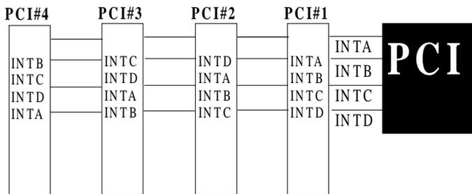
**Figure 7: The Combination of PCI INT#lines**
