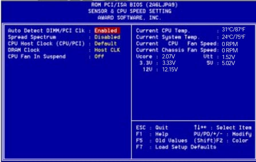
**Auto Detect DIMM/PCI Clk:** When enabled the motherboard will automatically disable the clock source for a DIMM socket which does not have a module in it. Same applies for PCI slots. The default is Enabled.
