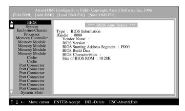
The four menus located on top of the DMI Configuration Utility screen are Edit DMI, Add DMI, Load DMI File and Save DMI File. Use the  $\leftarrow$  or  $\rightarrow$  (left or right) arrow keys to select a menu from the Menu bar.
