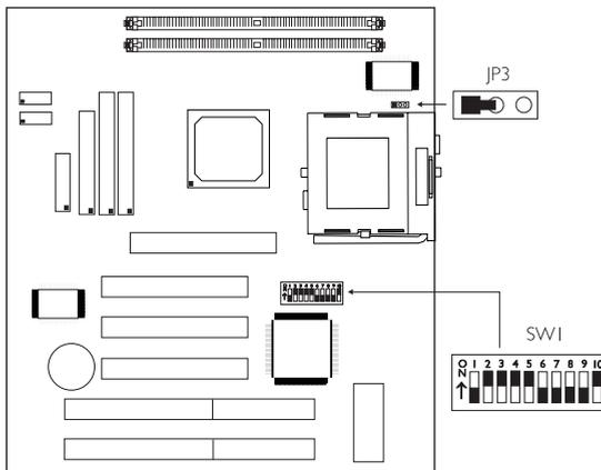
DIP Switch Settings for Intel Processors
