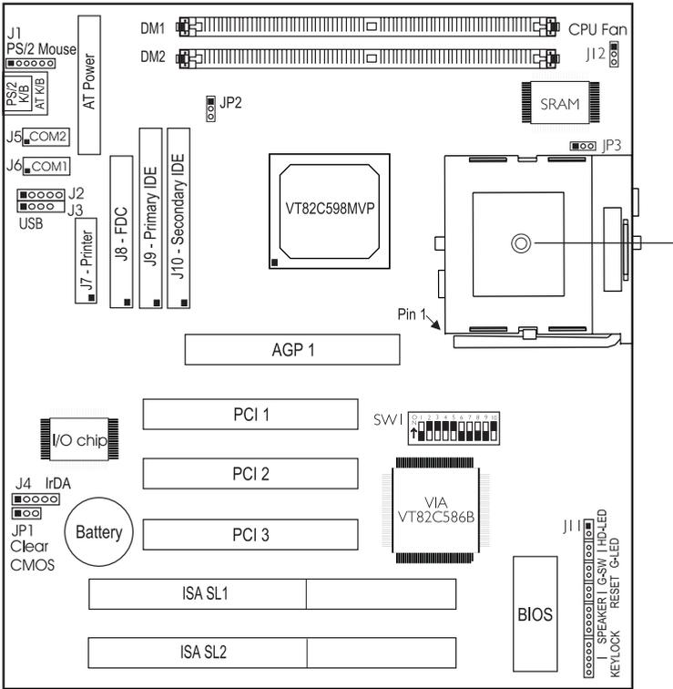
Mounting hole used for installing a mounting screw to secure the system board to the chassis.
