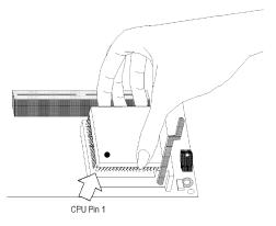
Positioning the CPU above the ZIF Socket
