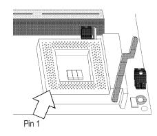
3 Position the CPU above the ZIF socket. Make sure pin 1 of the CPU is aligned with pin 1 of the socket. Lower the chip until the pins are inserted properly in their corresponding holes. Remember that very little force is needed to install the CPU. If the CPU is not easily inserted, verify whether or not pin 1 of the CPU is aligned with pin 1 of the socket. Applying too much pressure can damage the CPU or the socket.
