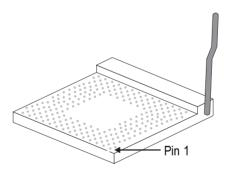
3. Position the CPU above the ZIF socket. Make sure pin 1 of the CPU is aligned with pin 1 of the socket. Lower the chip until the pins are inserted properly in their corresponding holes. Remember that very little force is needed to install the CPU. If the CPU is not easily inserted, verify whether or not pin 1 of the CPU is aligned with pin 1 of the socket. Applying too much pressure can damage the CPU or the socket.
