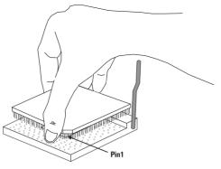
Positioning the CPU Above the ZIF Socket
