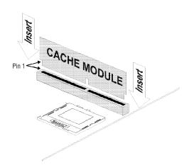
2. Once the cache module has been installed, make sure the "External Cache" option in the BIOS Features Setup menu of the Award PnP BIOS CMOS Setup Utility is set to "Enabled".
