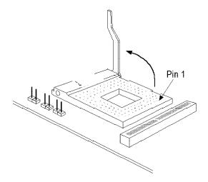
2. Once the lever is completely up, remove the old CPU by carefully lifting it straight out of the socket. You are now ready to insert the new CPU.
