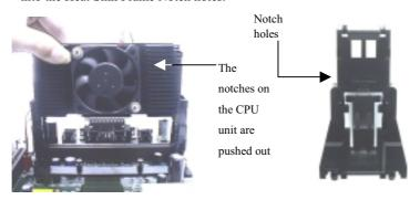
(2) Firmly secure the Heat Sink by attaching the Heat Sink Frame TOP-Bar. Please verify that the Heat Sink and CPU are tightly pressed together. Please check that the entire Frame, Heat Sink, and CPU unit are tightly installed and that there is no possible movement or looseness in the assembly.
