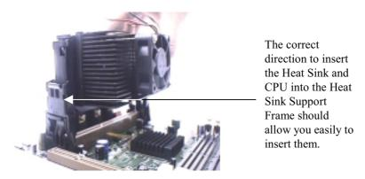
(2) Pushing the CPU unit into the frame, and waiting until the CPU unit is firmly in position before securing. The notches are pushed out. They will fit tightly into the Heat Sink Frame Notch holes.
