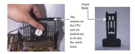
(3) Firmly secure the Heat Sink by attaching the Heat Sink Frame TOP-Bar. Please verify that the Heat Sink and CPU are tightly pressed together. Please check that the entire Frame, Heat Sink, and CPU unit are tightly installed and that there is no possible movement or looseness in the assembly.
