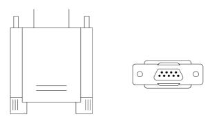
The serial ports on this system have two types of connectors, one 9-pin and one 25-pin. Some older computer systems and peripherals may only have a 25-pin connector. Should you need to connect your 9-pin serial port to a 25-pin serial port, you can purchase a 9-to-25 pin adapter.
