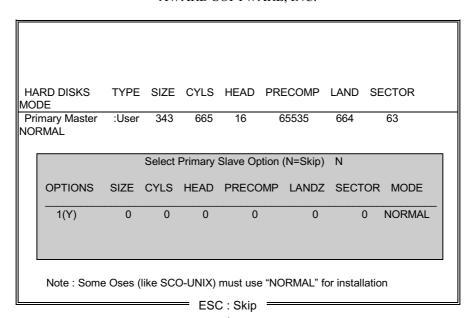
When you enter this utility, the screen asks you to select a specific hard disk for Primary Master. If you accept a hard disk detected by the BIOS, you can enter "Y" to confirm and then press <Enter> to check next hard disk. This function allows you to check four hard disks and you may press the <Esc> after the <Enter> to exit this function and go back to the Main Menu.
