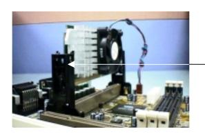
The correct direction to insert the Heat Sink and CPU into the Heat Sink Support Frame should allow you to easily insert them. (2) Pushing the CPU unit into the frame, wait until the CPU unit is firmly in position before securing. The notches are pushed out. They will fit tightly into the Heat Sink Frame Notch holes.
