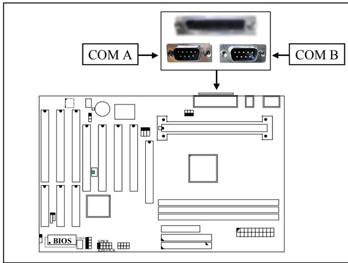
**Ping assignment of serial port connector:**
