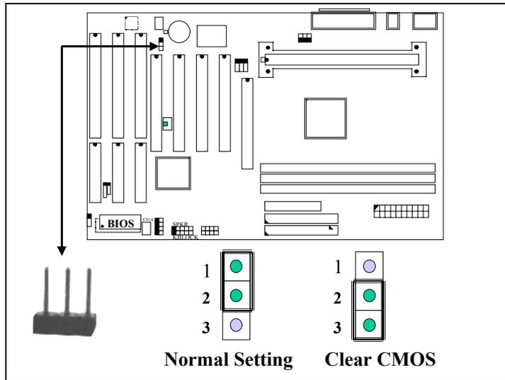
*Note: Improper BIOS setting may cause hang-up to the PC system, Should it be happened, you can use JP4 to clear the information which is stored in the CMOS memory and get the PC system back to normal. Improper connection may cause permanent damage to the mainboard. Please refer to the following steps to clear the CMOS*
