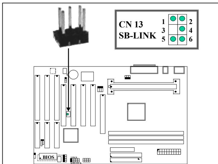
**Pin assignment of SB-LINK Connector:**
