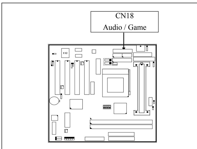
In order to have the audio device connected to the Audio Game port, an adapter is required. Please refer to the following picture for the connections on the adapter
