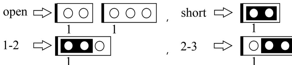
*The following jumpers which labeled with “optional” means they are the optional choice for customers and the related components are normally not populated on the mainboard. In order to make the mainboard works properly in your PC system, please make sure all jumper settings are at correct before installing this mainboard.*
