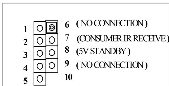
**3.3.14 CN13: CPU Cooling Fan Power Connector (FAN1)**
