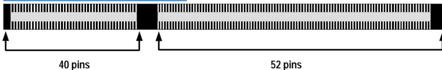
**Important: The DIMM's can only be fitted into the slots in one orientation. Make sure that the DIMM's are in the correct orientation and the pins are correctly aligned before you insert them.**
