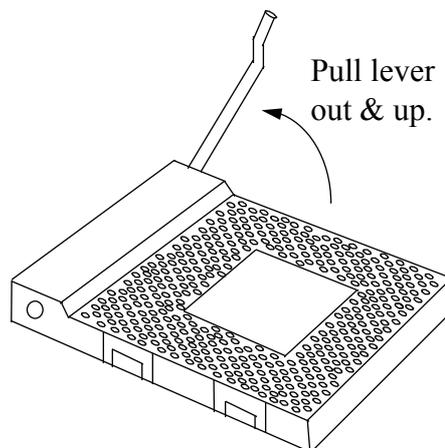
2. Align the CPU and socket pin 1 corners. Match the processor corner containing the blunt edge and the white dot to the socket corner with the distinctive pin arrangement. The pins on the bottom should have aligned with the inner 3 rings of holes in the socket. Place the CPU into the socket and it will go into the socket easily. If it won't, pull the level up a little more and try again.
