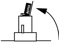
Push the SIMM module forward onto the positioning pins.
