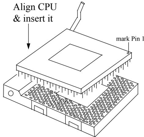
3. Press the lever down. The plate will slide forward. You will feel some resistance as the pressure starts to secure the CPU in the socket. When the CPU is installed, the lever will snap into place at the side of the socket.
