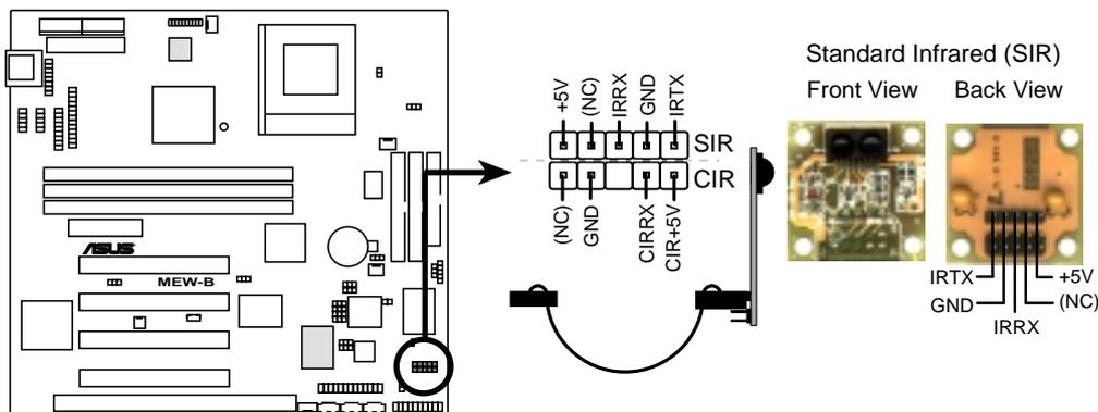
**MEW-B Infrared Module Connector**
