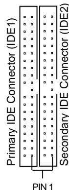
**NOTE:** Orient the red markings (usually zigzag) on the IDE ribbon cable to PIN 1
