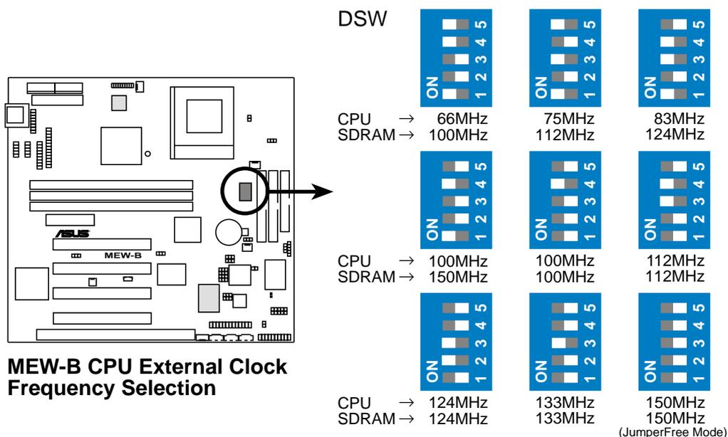
**NOTE:** Frequency Multiple settings are not available here because usually Socket 370 processors have locked Frequency Multiples. If your Socket 370 processor does not have a locked Frequency Multiple, you must use **CPU Core:Bus Freq. Multiple** in *4.4 Advanced Menu* of the BIOS setup to set the Frequency Multiple. If the Frequency Multiple is locked, setting the Frequency Multiple in BIOS setup will have no effect.
