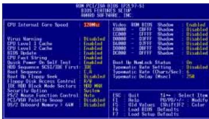
A section at the lower right of the screen displays the control keys you can use. Take note of these keys and their respective uses. If you need information on a particular entry, highlight it and then press <F1>. A pop-up help menu will appear to provide you with the information you need. <F5> loads the last set values, <F6> and <F7> loads the BIOS default values and Setup default values, respectively.
