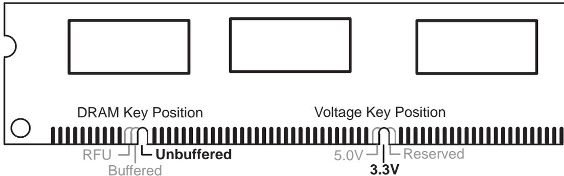
The notch on the DIMM module will shift between left, center, or right to identify the type and also to prevent the wrong type to be inserted into the DIMM slot on the motherboard. You must ask your retailer for the specifications before purchasing. Four clock signals are supported on this motherboard.
