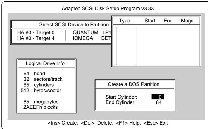
The Create a DOS Partition window suggests that you create one partition on the disk device, equal to its entire capacity. If this is what you want to do, skip to step 5.
