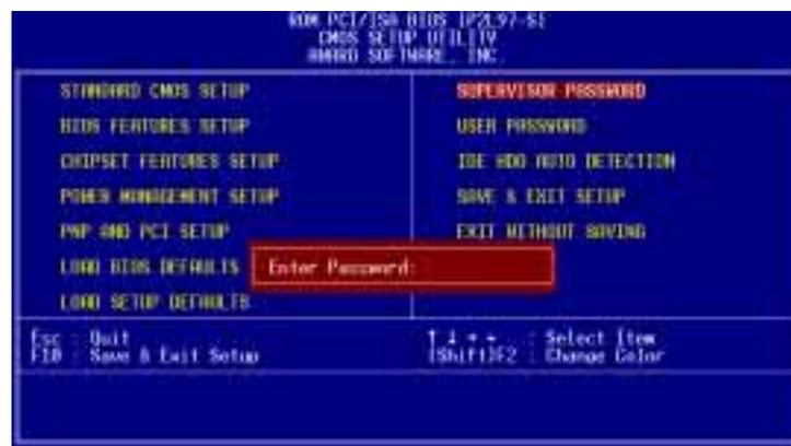
To implement password protection, specify in the “Security Option” field of the BIOS Features Setup screen when the system will prompt for the password. If you want to disable either password, press <Enter> instead of entering a new password when the “Enter Password” prompt appears. A message confirms the password has been disabled.
