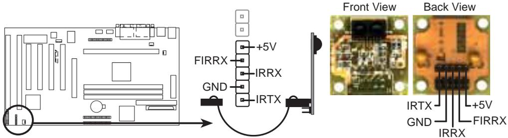
**Infrared Module Connector**
