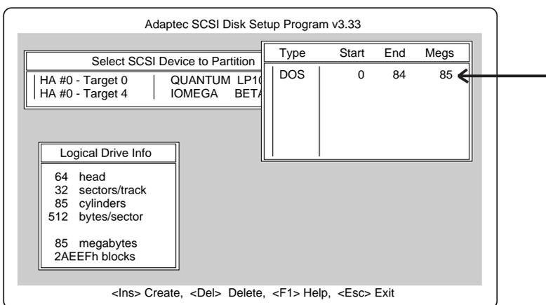
6. Press Esc to return to the Select SCSI Device to Partition window. If you want to partition a different disk device, select the device from the list and repeat the earlier steps.
