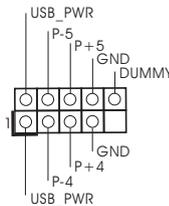
ASRock I/O™ provides you 4 default USB 2.0 ports on the rear panel. If the rear USB ports are not sufficient, this USB 2.0 header is available for 2 additional USB 2.0 ports.
