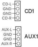
These connectors allow you to receive stereo audio input from sound sources such as a CD-ROM, DVD-ROM, TV tuner card, or MPEG card.
