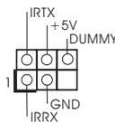
This connector supports an optional wireless transmitting and receiving infrared module.
