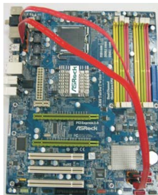
Connect the SATA data cables to both orange eSATAII connectors (eSATAII_BOTTOM and eSATAII_TOP)
