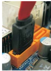
Connect the SATA data cable to one of the orange eSATAII connector (eSATAII_BOTTOM)
