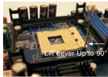
STEP 1: Lift The Socket Lever Up to 90°
