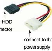
Please connect the black end of SATA power cable to the power connector on the drive. Then connect the white end of SATA power cable to the power connector of the power supply.
