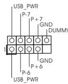
ASRock I/O Plus™ provides you 6 ready-to-use USB 2.0 ports on the rear panel. If the rear USB ports are not sufficient, this USB 2.0 header is available to support 2 extra USB 2.0 ports.
