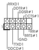
This COM1 connector supports a serial port module.
