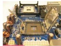
Step 1-3. Rotate the load plate to fully open position at approximately 100 degrees.
