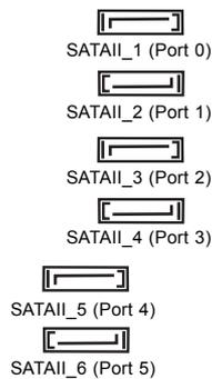
These six Serial ATAII (SATAII) connectors support SATA data cables for internal storage devices. The current SATAII interface allows up to 3.0 Gb/s data transfer rate.
