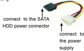
Please connect the black end of SATA power cable to the power connector on each drive. Then connect the white end of SATA power cable to the power connector of the power supply.
