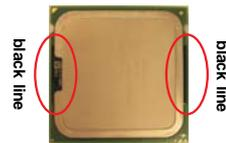
Step 2-2. Orient the CPU with IHS (Integrated Heat Sink) up. Locate Pin1 and the two orientation key notches.
