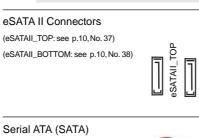
These two eSATA II connectors support SATA data cables for external SATAII function. The current eSATA II interface allows up to 3.0 Gb/s data transfer rate.
