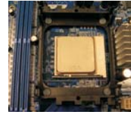
STEP 4: Push Down And Lock The Socket Lever
