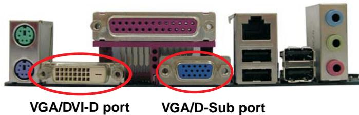
2. If you have installed onboard VGA driver from our support CD to your system already, you can freely enjoy the benefits of dual monitor function provided by VGA/DVI-D and VGA/D-Sub ports with this motherboard after your system boots. If you haven't installed onboard VGA driver yet, please install onboard VGA driver from our support CD to your system and restart your computer. Then you can start to use dual monitor function provided by VGA/DVI-D and VGA/D-Sub ports with this motherboard.
