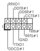
This COM1 header supports a serial module.
