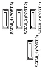
These four Serial ATAII (SATAII) connectors support SATAII or SATA hard disk for internal storage devices. The current SATAII interface allows up to 3.0 Gb/s data transfer rate.
