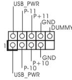
Besides four default USB 2.0 ports on the I/O panel, there are four USB 2.0 headers on this motherboard. Each USB 2.0 header can support two USB 2.0 ports.
