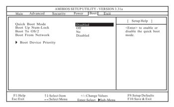
Quick Boot Mode: Enable this mode will speed up the boot-up routine by skipping memory retestings.
