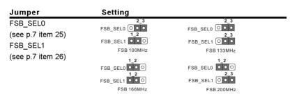
Note: The setting of the CPU front side bus frequency of this motherboard is by means of the adjustment of jumper-setting. Please follow the figures above to set the CPU front side bus frequency. Please note that the setting of FSB 200MHz will function only when the installed CPU supports FSB 200MHz.
