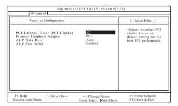
PCI Latency Timer (PCI Clocks): The default is 32. It is recommended to keep the default value unless the installed PCI expansion cards' specifications require other settings.
