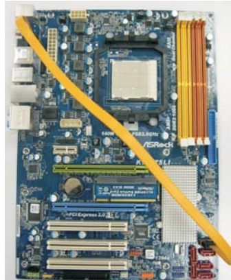
Connect the SATA data cable to the eSATAII connector (eSATAII_TOP)
