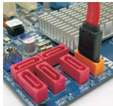
Connect the SATA data cable to the orange SATAII connector (SATAII_6 (PORT5))
