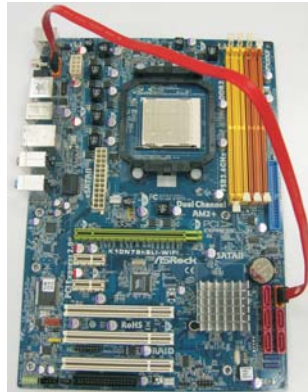
Connect the SATA data cable to the eSATAII connector (eSATAII_TOP)
