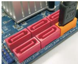
Connect the SATA data cable to the orange SATAII connector (SATAII_6 (PORT5))
