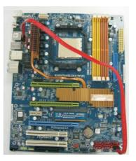
Use the eSATAII device cable to connect eSATAII device and the eSATAII port of the I/O shield according to the eSATAII connector that you connect the SATA data cable.
