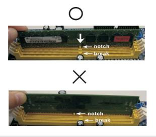
The DIMM only fits in one correct orientation. It will cause permanent damage to the motherboard and the DIMM if you force the DIMM into the slot at incorrect orientation.
