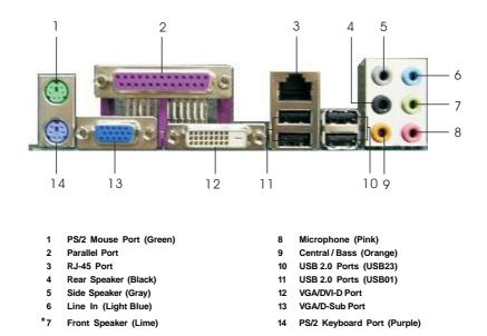
\* If you use 2-channel speaker, please connect the speaker's plug into "Front Speaker Jack". See the table below for connection details in accordance with the type of speaker you use.
