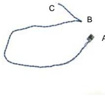
Please connect the black end (A) of HDMI\_SPDIF cable to the HDMI\_SPDIF header on the motherboard. Then connect the white end (B or C) of HDMI\_SPDIF cable to the HDMI\_SPDIF connector of HDMI VGA card.
