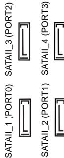
These four Serial ATAII (SATAII) connectors support SATA data cables for internal storage devices. The current SATAII interface allows up to 3.0 Gb/s data transfer rate.
