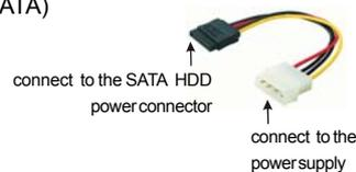
Please connect the black end of SATA power cable to the power connector on each drive. Then connect the white end of SATA power cable to the power connector of the power supply.
