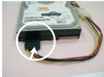
**Step 4** Connect SATA data cable to the SATA / SATAII HDD.
