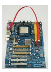
2. Use the eSATAII device cable to connect eSATAII device and the eSATAII port of the I/O shield.
