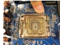
Step 1-2. Rotate the load lever to fully open position at approximately 135 degrees.
