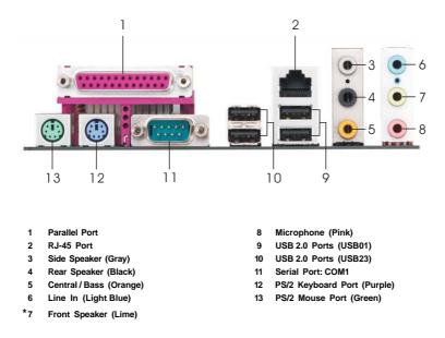
\* If you use 2-channel speaker, please connect the speaker's plug into "Front Speaker Jack". See the table below for connection details in accordance with the type of speaker you use.
