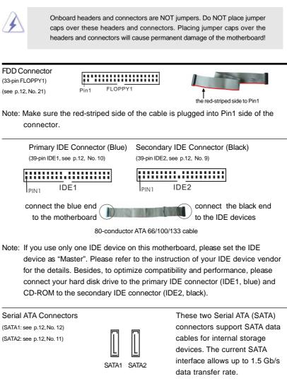
Serial ATA (SATA) Data Cable Either end of the SATA data cable can be connected to the SATA hard disk or the SATA connector on the motherboard.
