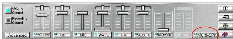
**Notice:** If users set Multi-SPK mode and connect only stereo speakers to Speaker jack on the front panel or Front Out jack on the back of PC, that will cause an incomplete audio output.
