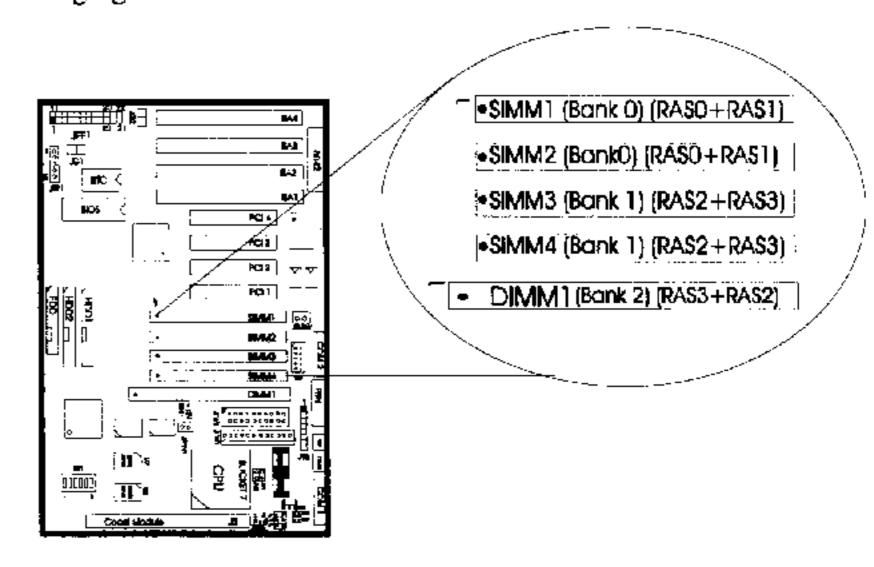
Warning! Memory bank 0 & 1's SIMM power level is 5 volts.
