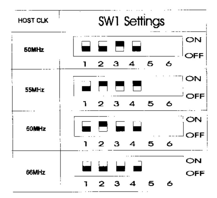
Note 2: Pins #5 and #6 of the DIP Switch SW1 are used to set the Core/Bus (Fraction) ratio of the CPU. The actual core speed of the CPU is the Host Clock Frequency multiplied by the Core/Bus ratio. For example:
