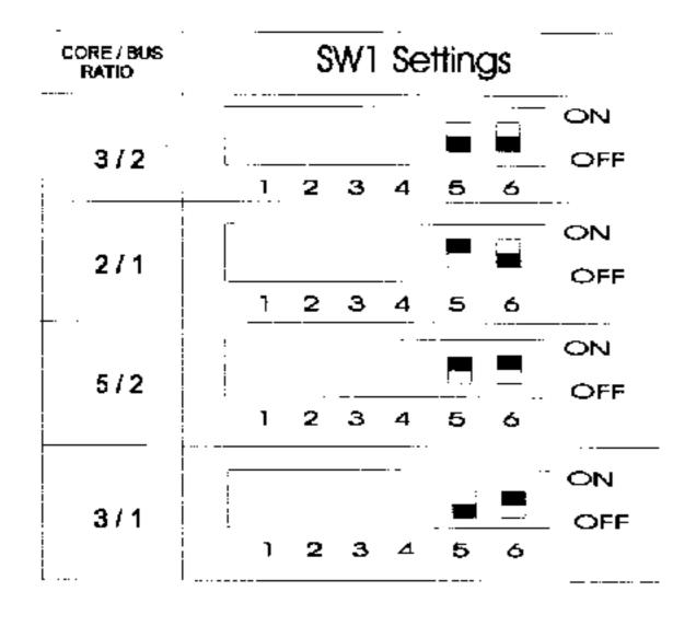
Note 3: The PCI Bus Clock is the Host Clock Frequency divided by 2.
