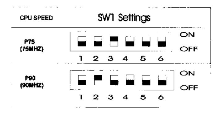
Note 1: The 4 Host Clock Frequencies that the system supports are 50MHz, 55MHz, 60MHz, and 66.6MHz.(By adusting pins 1,2,3,and 4 of SW1 the Host Clock Frequency can be selected). See the following chart to set the different Host Clock frequencies.
