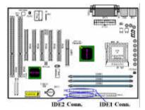
An IDE hard disk drive ribbon cable has 40 wires and two connectors to provide a connection for two IDE hard disk drives. After connecting the single end to the IDE1 (or IDE2), connect the two connectors on the other end to the IDE hard disk drives (or CD-ROM drive, LS-120, etc.).
