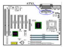
Attach the connector from the power supply to the ATX1 connector here. Remember you have to push the connector from the ATX power supply firmly to the end with the ATX1 connector, insuring that you have a good connection.
