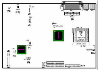
Figure 2-7. All Connectors and Headers for the ZM6
