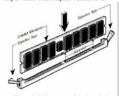
Figure 2-6. Memory module installation
