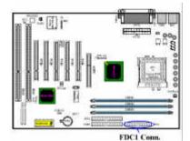
This 34-pin connector is called the "floppy disk drive connector". You can connect a 360K, 5.25", 1.2M, 5.25", 720K, 3.5", 1.44M, 3.5" or 2.88M, 3.5" floppy disk drive, you can even connect a 3 Mode floppy disk drive (it's a 3 1/2" drive used in Japanese computer systems).
