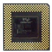
Figure 1-1. Intel® Celeron ™PPGA package processor
