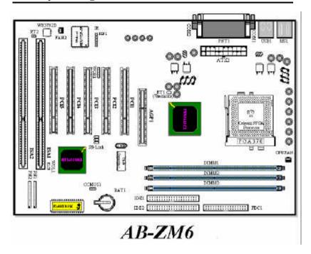
Figure 1-2. Motherboard component location
