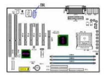
There is a specific orientation for pins 1 through 5, attach the connector from the IR KIT or IR device to the IR header. This motherboard supports standard IR transfer rates.
