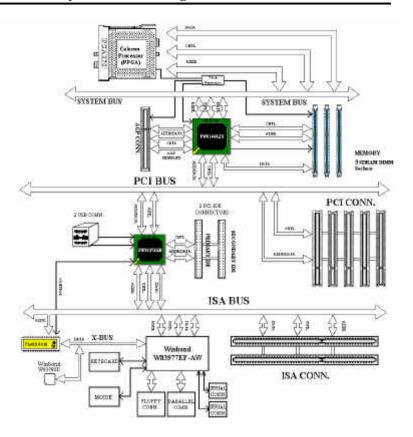
Figure 1-3. System diagram of the 440ZX chipset
