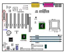
This slot is used for an optional CNR with the main objective of reducing the baseline implementation cost of features that are widely used in the "Connected PC", while also addressing specific functional limitations of today's audio, modem, and LAN subsystems.
