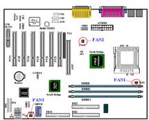
(2A)/(2B)/(2C): FAN1, FAN2 & FAN3 header
