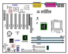
This header is reserved for system management bus (SM bus). The SM bus is a specific implementation of an  $I^2C$  bus.  $I^2C$  is a multimaster bus, which means that multiple chips can be connected to the same bus and each one can act as a master by initiating a data transfer. If more than one master simultaneously tries to control the bus, an arbitration procedure decides which master gets priority.
