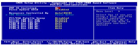
Figure 3-9. PnP/PCI Configurations Setup Screen Shot
