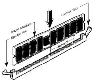
Figure 2-4. Memory module installation
