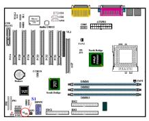
This header is for the connection of chassis intrusion detection.
