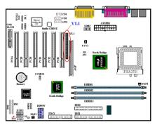
This connector is used for inserting an optional add-on card to enable the on board VGA to be output to TV-Out or Flat Panel.
