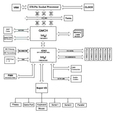
Figure 1-2. System diagram of the INTEL 815E Chipset
