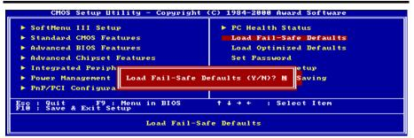
Figure 3-12. Load Fail-Safe Defaults Screen Shot
