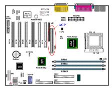
This function is used for installing an AGP Inline Memory Module (optional model RM-04). This is an optional feature to improve the on board VGA by enhancing the 3D performance.
