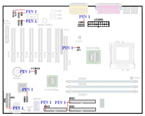
Figure 2-5. All Connectors and Headers for the SE6
