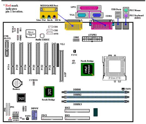
Figure 1-1. SE6 Motherboard component location
