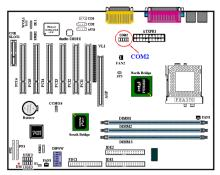
You can have one additional COM2 plugs affixed to the back panel by attaching an expansion cable that comes with the motherboard. Please align the red line of the cable to the pin 1 of COM2 header.
