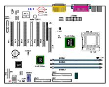
This header is for the internal CD-ROM drive audio cable connection. Please check your audio cable attached with the CD-ROM drive to see which type of connector you have and then plug it into this header.
