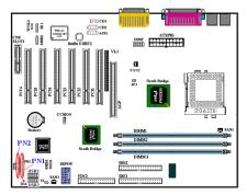
PN1 and PN2 are for switches and indicators of the chassis' front panel. There are several functions that come from these two headers. You have to watch the pin position and the orientation, or you may cause system malfunctions. Figure 2-7 shows you the functions of PN1 and PN2.
