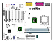
If you have a network adapter that supports this feature, then you can connect the specific cable from the network adapter to this header. This feature lets you wake up your computer via remote control through a local area network. You may need a specific utility to control the wake up event, such as the PCnet Magic Packet utility or other similar utilities.
