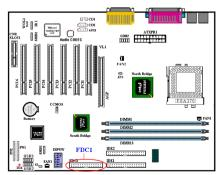
This 34-pin connector is called the "*floppy disk* drive connector". You can connect a 360K, 5.25", 1.2M, 5.25", 720K, 3.5", 1.44M, 3.5" or 2.88M, 3.5" floppy disk drive. You can even connect a 3 Mode floppy disk drive (a 3 1/2"
