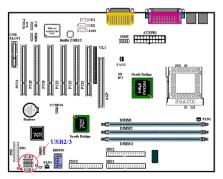
These headers are used for connecting the additional USB ports plug. You can have two additional USB plugs affixed to the back panel
