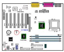
The jumper CCMOS discharges CMOS memory. When you install the motherboard, make sure this jumper is set for normal operation (pin 1 and 2 shorted). See figure 2-6.
