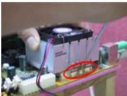
Check the photo on the left. You have finished the heatsink installation.
