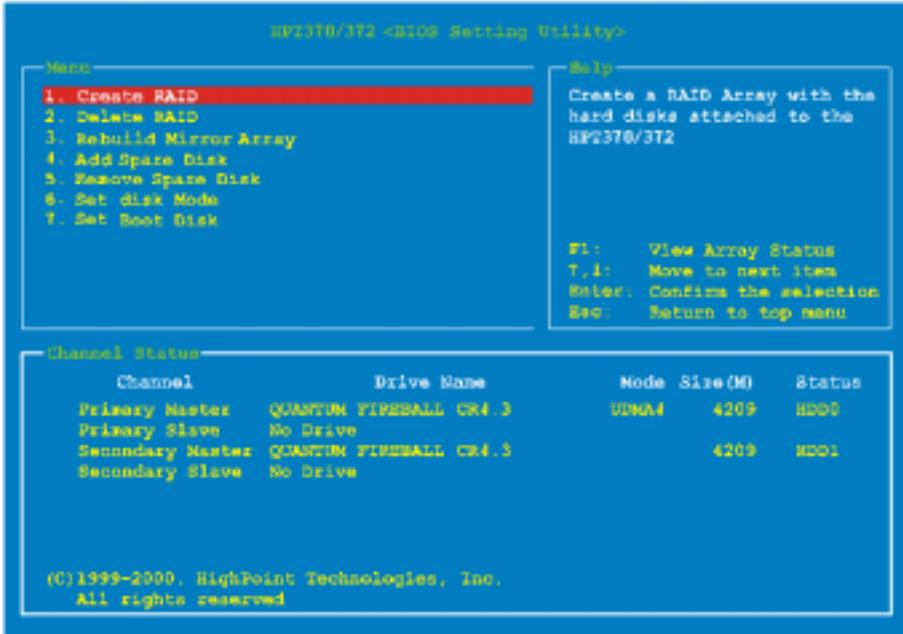
Reboot your system. Press <CTRL> and <H> key while booting up the system to enter the BIOS setting menu. The main menu of BIOS Setting Utility appears as below:
