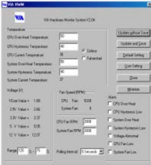
This screen shows the VIA hardware monitor system screen. It displays information about system temperature, voltages, and fan speed. Some items allow you to set the warning range; you can adjust your system to optimize the value settings.
