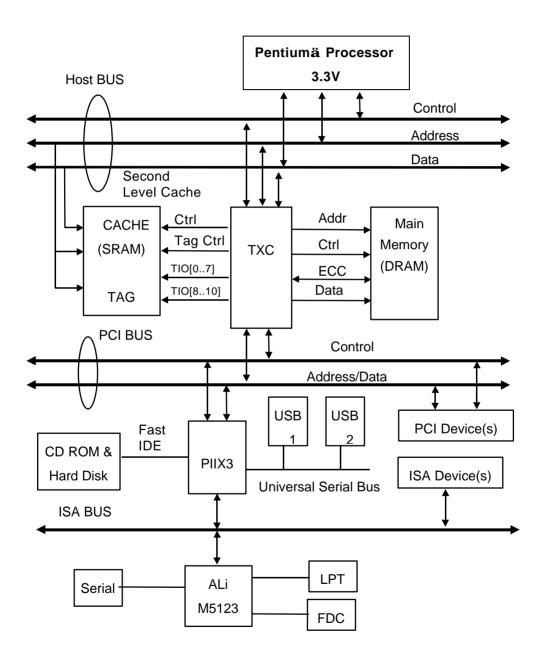
Fig. 1-4 System block diagram
