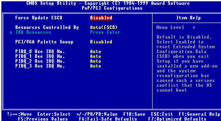
Figure 3-9. PnP/PCI Configurations Setup Screen Shot
