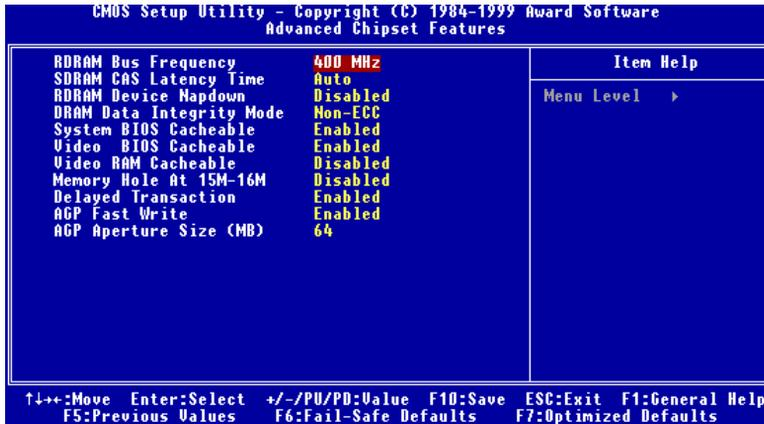
Figure 3-6. Advanced Chipset Features Setup Screen Shot
