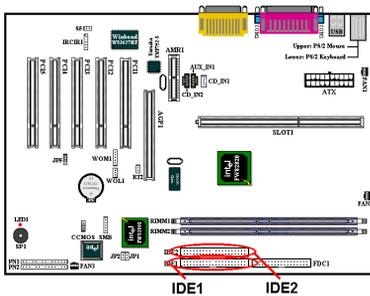
An IDE hard disk drive ribbon cable has 40 wires and two connectors to provide a connection for two IDE hard disk drives. After connecting the single end to the IDE1 (or IDE2), connect the two connectors on the other end to the IDE hard disk drives (or CD-ROM drive, LS-120, etc.).
