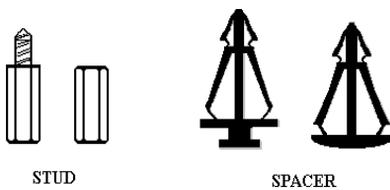
Figure 2-1. The outline of stub and spacer
