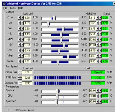
**Step 6.** This screen will appear. You will see voltages, fan speeds and temperature readings as well. If any item readings are critical or over their limitations, the reading will turn red. Also, a pop-up window will appear to warn you the system has a problem!
