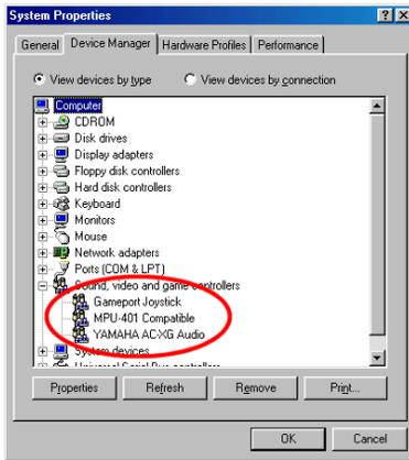
Once Windows has restarted, go to "System Properties" to double check. You should find the "? PCI Multimedia Audio Device" has disappeared, and Yamaha AC-XG audio Codec is there instead.
