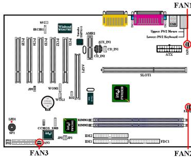
Attach the connector from the individual CPU fan to the header named FAN2, and attach the connector from the chassis fan to FAN3 or FAN1 header.
