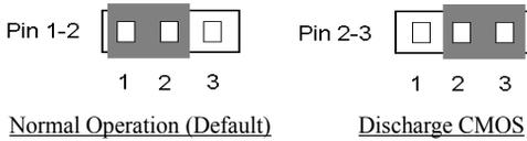
Figure 2-7. CCMOS1 jumper setting
