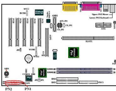
PN1 and PN2 are for switches and indicators for the chassis's front panel, there are several functions that come from these two headers. You have to watch the pin position and the orientation, or you may cause system malfunctions. Figure 2-8 shows the PN1 and PN2 functions of the pins.
