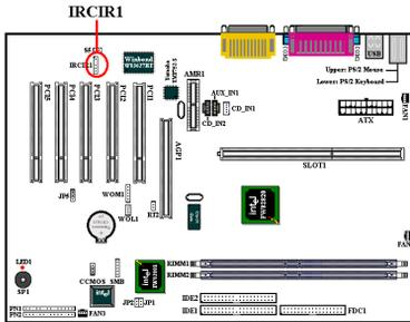
There is a specific orientation for pins 1 through 5, attach the connector from the IR KIT or IR device to the IRCIR1 header. This motherboard supports standard IR transfer rates.
