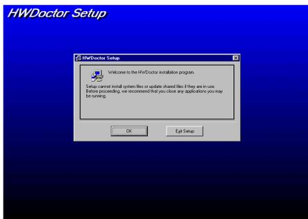
**Step 1.** In Windows<sup>®</sup> 95/98, place the CD-ROM into the computer. The main menu will appear. Click the **Hardware Doctor Install** button. The *HWDoctor Setup* screen will show up. Please refer to the figure below.
