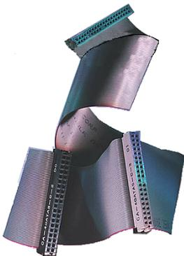
**Figure 2-10. Photo of an Ultra ATA/66 Conductor**
