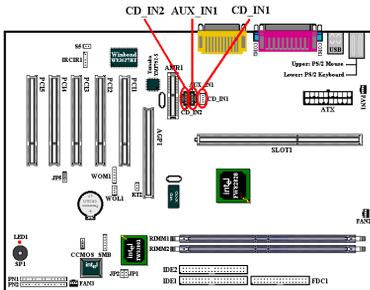
**AUX\_IN1:** This connector is used for other internal audio cable connections. For example, if you have installed two internal CD-ROM drives in your computer system, you can connect a secondary CD-ROM drive audio cable to this connector.
