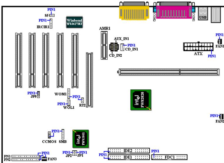
Figure 2-6. All Connectors and Headers for the CX6
