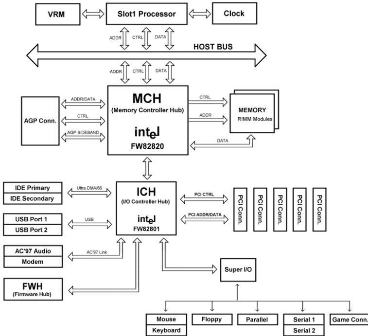
Figure 1-2. System diagram of the Intel 820 chipset
