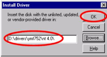
You have to specify and manually type the path of driver location. We've put the audio drivers under the "DRIVERS\YMF752\NT4.0". The code name of the CD-ROM drive will depend on how many devices installed on your computer system. Here it is shown as D:\.
