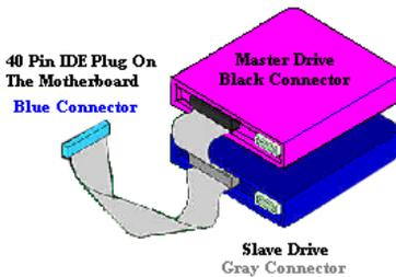
**Figure 2-11. How to connect an ATA/66 Cable to the Motherboard**
