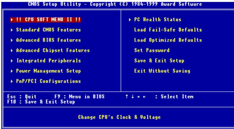
**Figure 3-1. CMOS Setup Utility Main Screen Shot**
