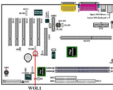
If you have a Network adapter that supports this feature, then you can connect the specific cable from the network adapter to this header. This feature lets you wake up your computer via remote control through a local area network. You may need a specific utility to control the wake up event, like using the Intel® LDCM® utility or other similar utilities.
