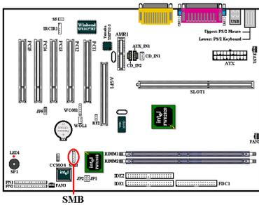
This connector is reserved for system management bus (SMBus). The SMBus is a specific implementation of an I<sup>2</sup>C bus. I<sup>2</sup>C is a multi-master bus, which means that multiple chips can be connected to the same bus and each one can act as a master by initiating a data transfer. If more than one master simultaneously tries to control the bus, an arbitration procedure decides which master gets priority.
