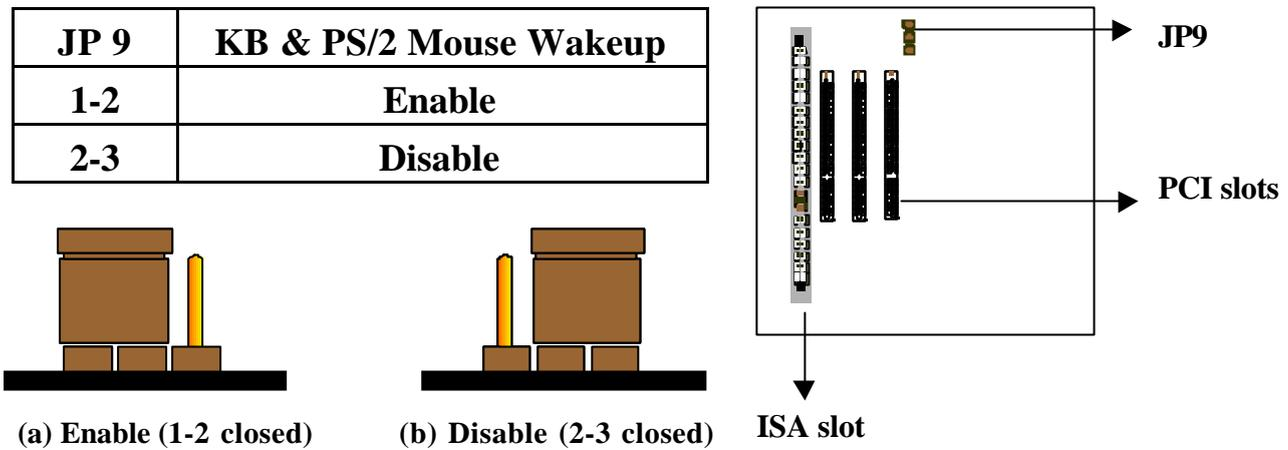
The default Power On function is “Button Only”. That means, we can only turn our computer on and off by pressing the “Power Button”. If we want to enable KB & PS/2 Mouse Power On function, we first have to set JP9 to Pin 1-2 closed, and then go to “Power On Function” in “Integrated Peripherals” of Award BIOS Setup. At the line “Power On Function”, we can press “Page Up” or Page Down” to make the following selections:
