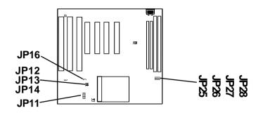
JP11, J12, J13, J14, JP16 - Power Selection for the CPU Core Voltage, Bus Section and Bus Voltage
