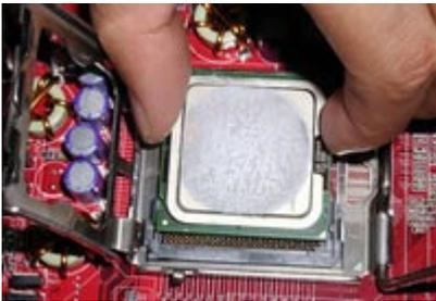
3. Use index finger and thumb to place the CPU onto the plastic body (look for the gold arrow on the CPU. The gold arrow should point away from the lever pivot).
