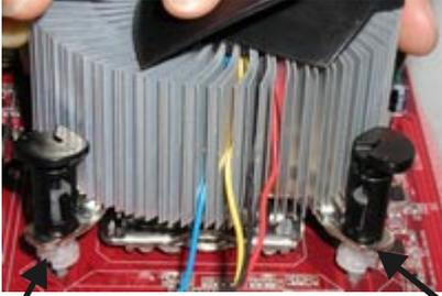
7. Align the fastener tips with the motherboard hole pattern, insert the fastener tips into the holes, guiding the wires to avoid pinching. The fasteners will slide through the motherboard holes with no insertion force.
